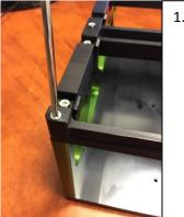
1.Remove 14X M3 countersunk Screws from Top of Diti Carrier
