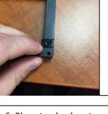
6. Place top back onto assembly and screw 14X M3 countersunk screws into holes.
